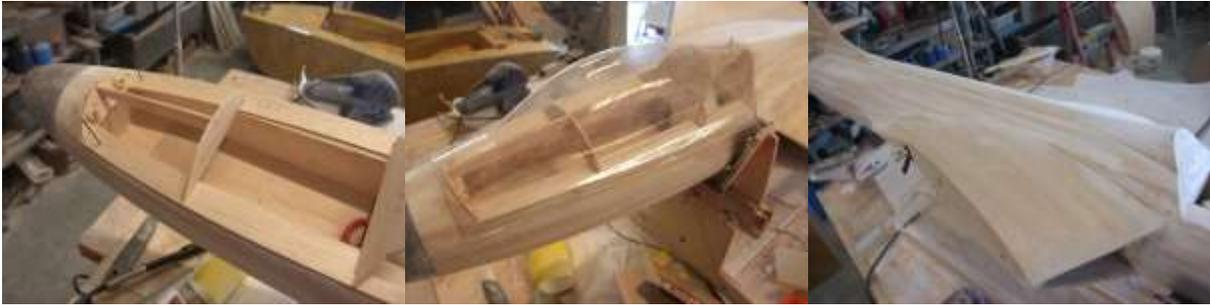
**Make the canopy fit to the frame and fuselage , cut oversize and make fit
