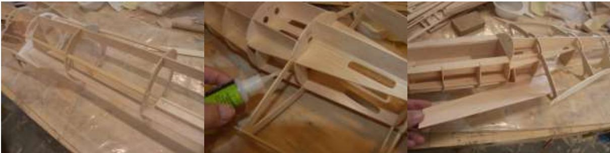
**Now place the duct lining ,cut as per plan from thick paper in 2 pieces , it can be done in 1 piece but it is a hard job.**
