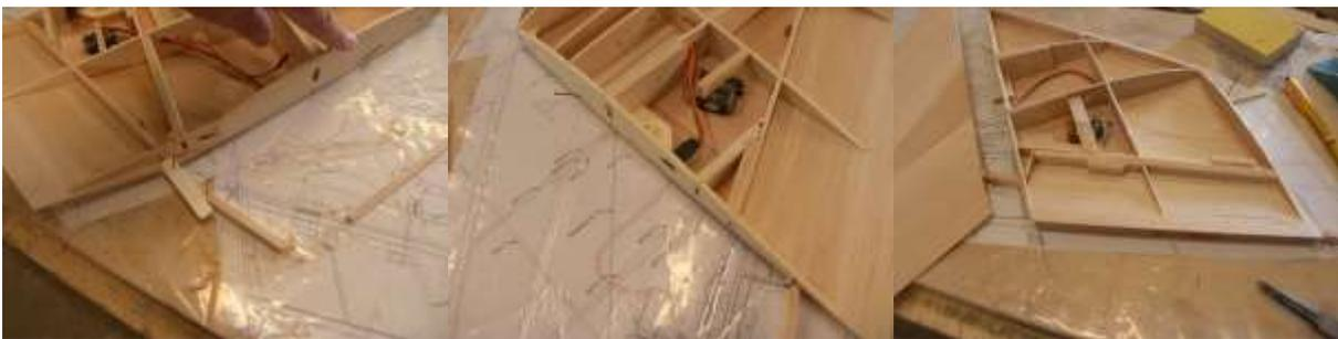
Cut the top sheeting , mark it with some lines from the inner panel as lead .
