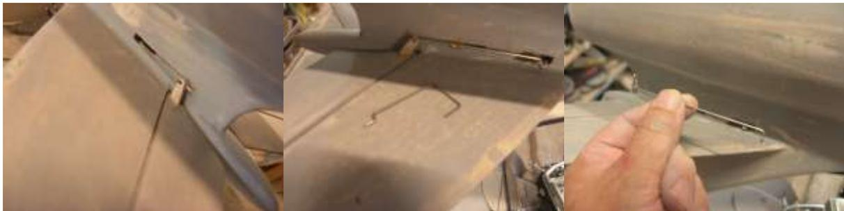
**Use 1,2 or 1,5mm steel wire make Z-bends both sides , solder other side to main steering wire with help from some wire or brass tube , make sure travel is the same and aligned, when all is satisfying then glue steering arms into elevators**
