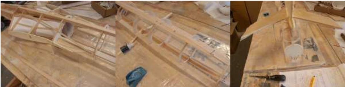
**Now nail down the fuselage assembly with help from some spare balsa scrap at the wing sections and tail section, btw better take out the inside of F42 before gluing to fuselage.**
