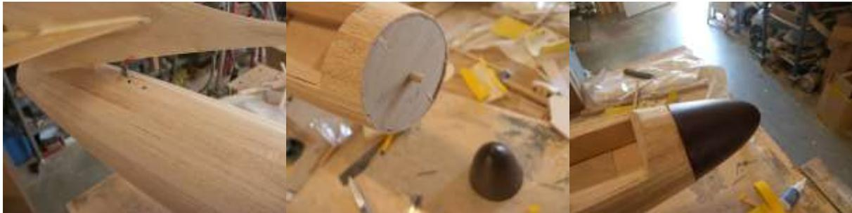
We finished the Hunter fuselage with thinned superlight filler , brush it on , sand with 60 grit, the glass the fuselage.
