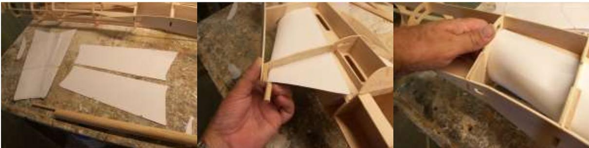
**When done place scrap 6x12mm balsa on the intake lips place 3x balsa on the ducts for strengthening as per plan.**
