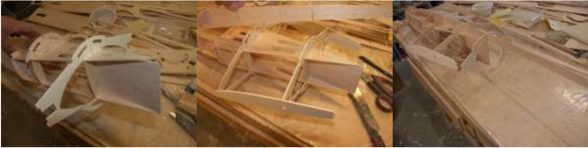
**Align Fuselage as much as you can and glue other parts with thin or medium ca.**
