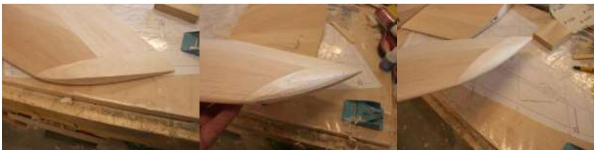
Join wing parts with spruce joiners outer panels have the joiners glued in, they slide into the inner panels.
