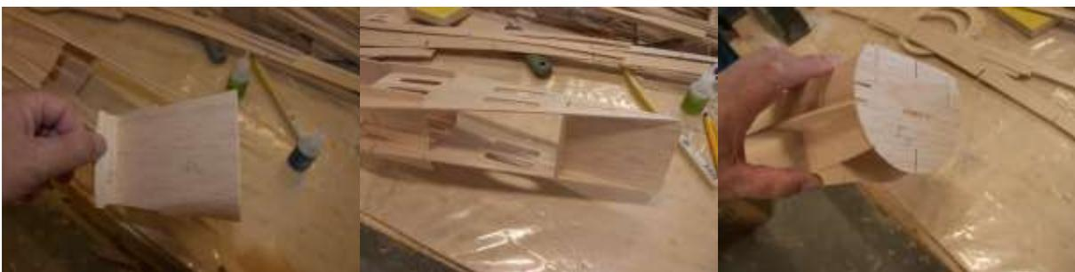
**You can glue most formers in the nose section with thin ca , do not glue F19 and F20 yet
