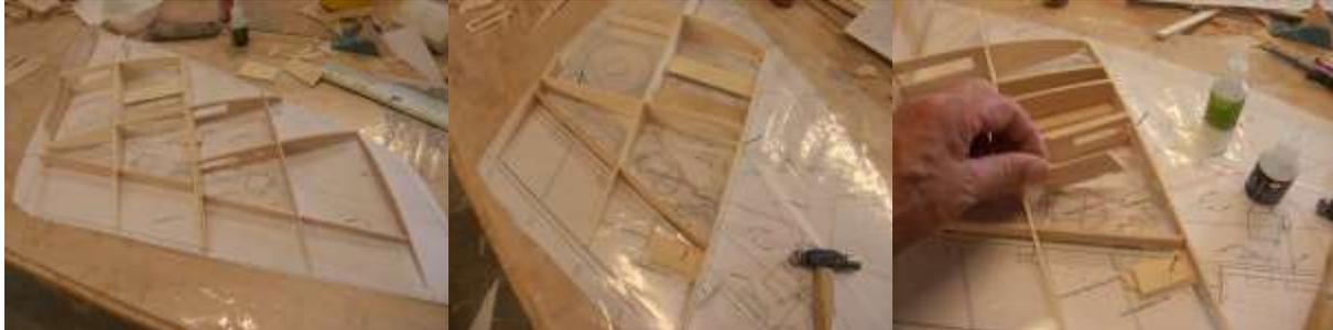
Make sure the parts are sliding in smooth , to tight a fit can warp the parts , so sand if necessary.
