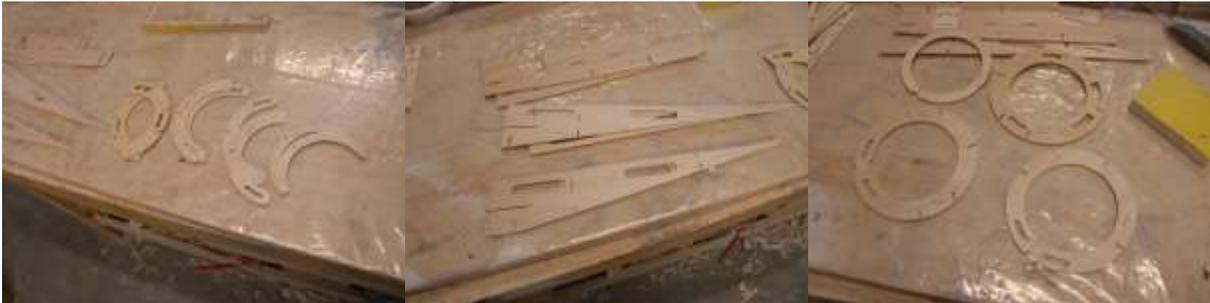
**Now start by adding formers to F11 , do not glue yet. The front part of the fuselage can almost complete done.**
