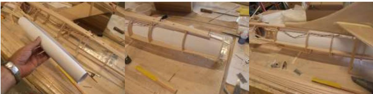
**When ducts are glued to the formers the fuselage is twist stiff so take care for alignment.**
