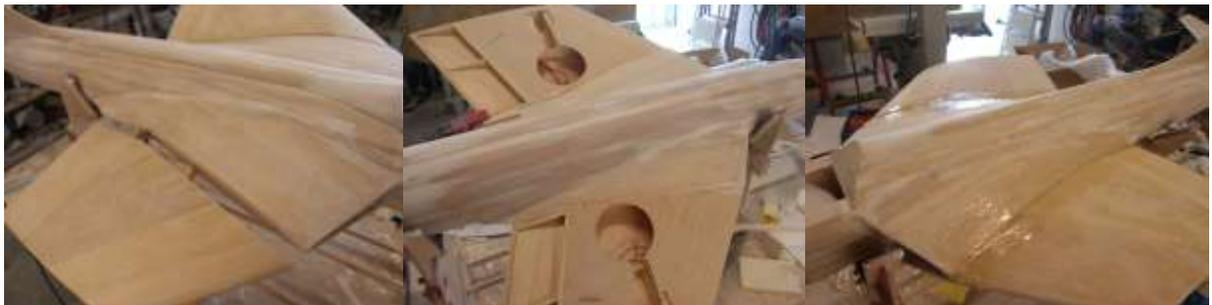
Glass the wing joint with epoxy and 120gr glass,
