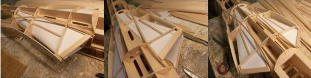
**Place 2x 2x12 sheet strip to bottom of fuselage use the centre former for aligning the strips.**
