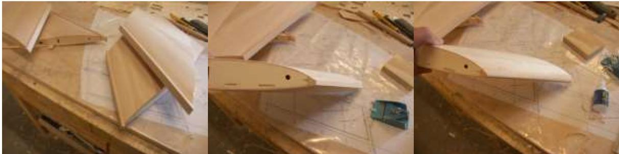
Join tip blocks and place to tip note that the leading edge at the tip curves a bit back so the tip should not be place at the front of the leading edge but a few (2)mm back sand tips with course paper and razorplane ,
