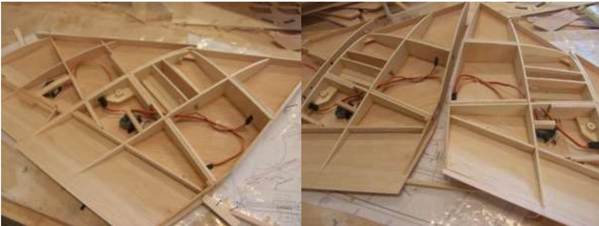
sand all so there are no high spots and pin down the inner panel to the building board with help from the 6x12 helpformer for the correct washout, pin down the wing at the X marked points.
