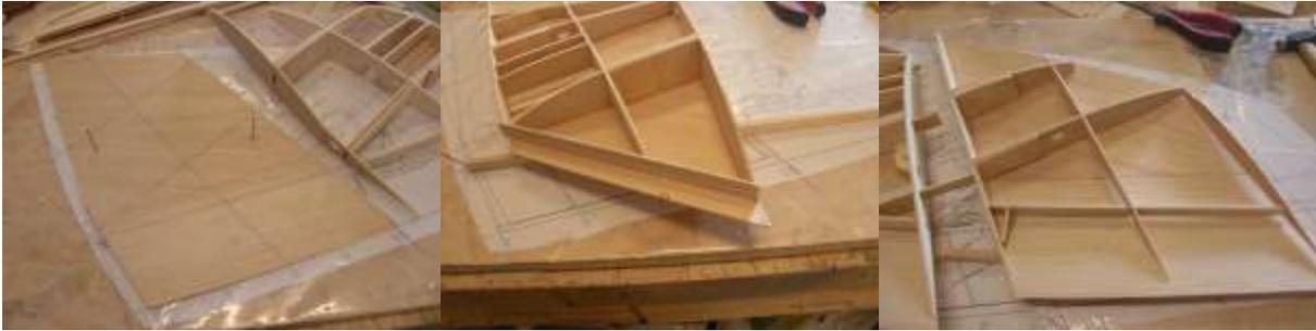
Make the wing joiner fastener from the M3 set and ring with help from M3x30 fastener glue to the wing joiner parts .Place the outer wing part with the Joiner into the inner part , make sure it slides easy , mark WJ1 with help from the M3 fastener , drill 3mm.
