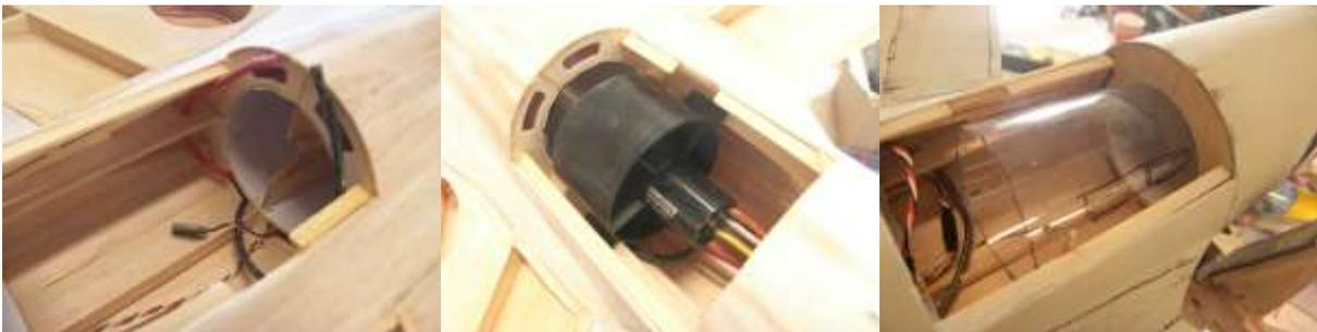
**Make the outlet tube from the supplied pvc sheet as per plan , do fit and try , we use cello tape to yoin the plastic, make openings for wiring , place tube into exhaust tube in fuselage , then slide forward over fan unit and fasten with tape ,**
