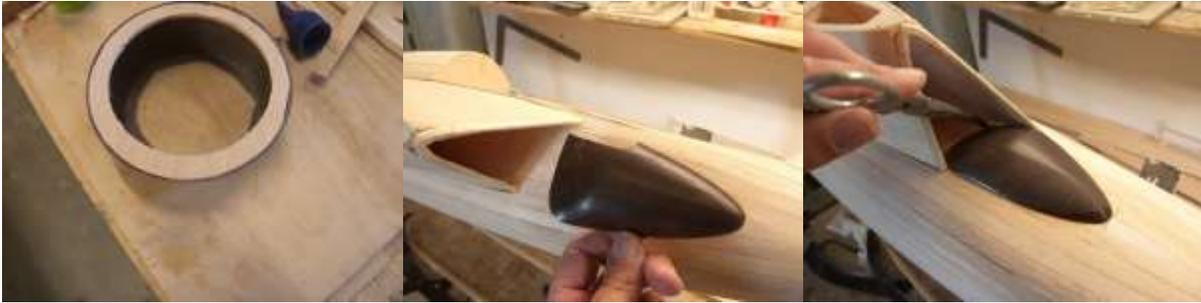
**Make canopy frame from formers as per plan, place top sheeting inside canopy from stiff paper. Clean opening in F17 for canopy closing , harden opening with thin ca. Carefully draw canopy edges with a sharpie better a bit too large as to small cut canopy and glue to frame with canopy glue, we use ca (clean up canopy with window cleaner first)**
