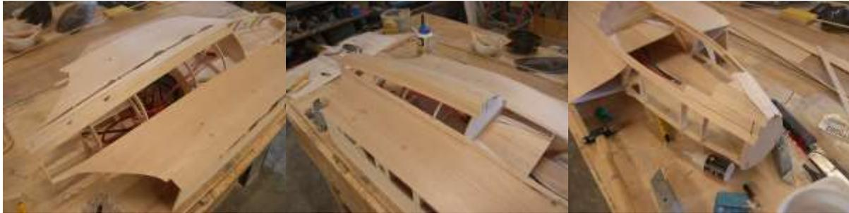
Turn over fuselage into build support, it will fit at the wing sections use some in between balsa , the fuselage is stiff now
