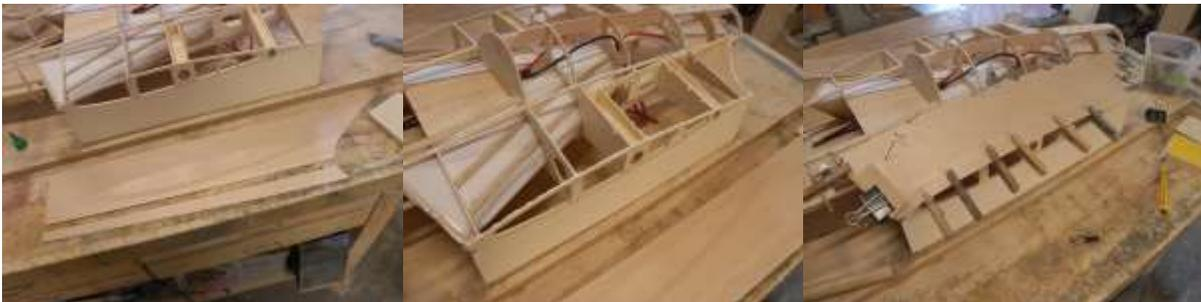
Place 2x 2x12 sheet strip to top of fuselage use the centre former for aligning the strips. Sand flat at rudder position and make openings for dowels and (we did not use a rudder but if you like you can add one) servo wire.
