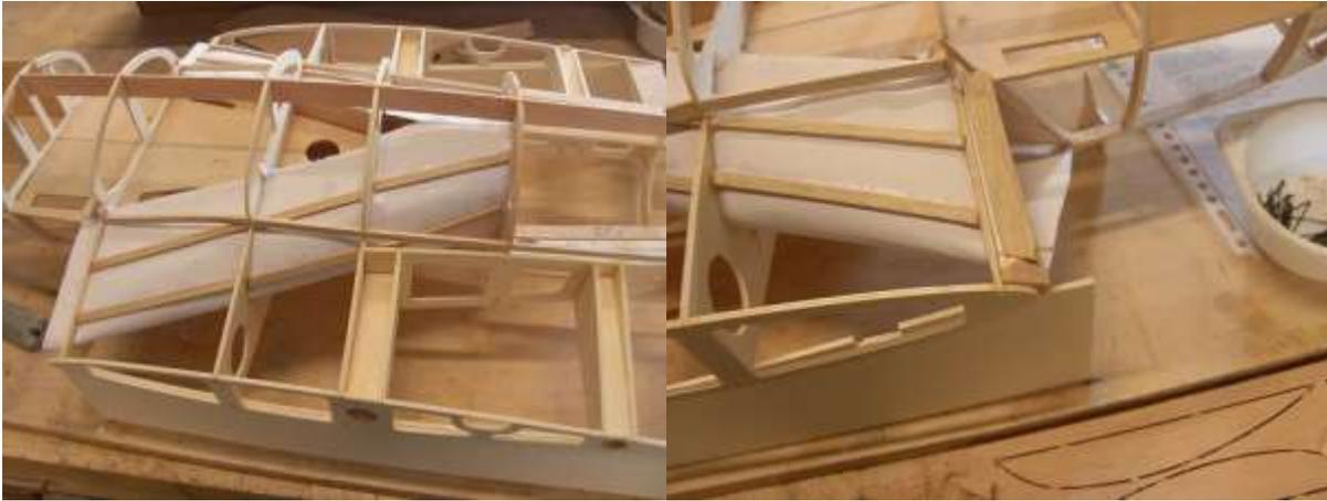
Place motor wiring and servo leads. Sand top of F23 flush to take fairing sheet, make sure fuselage is straight and level with fuselage build support place build support formers in front and back see pictures on cd, place 3x6 stringers
