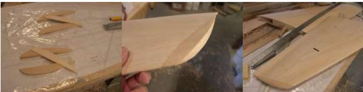
**Take out opening for your retracts, use some scrap ply to fill the mount till the top of the retract unit is flush with the wing sheeting**
