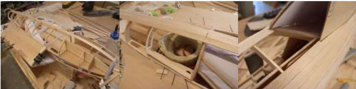
**Mark front retract hatch , you can make a working hatch or make a tight fit hatch around the retract leg.**
