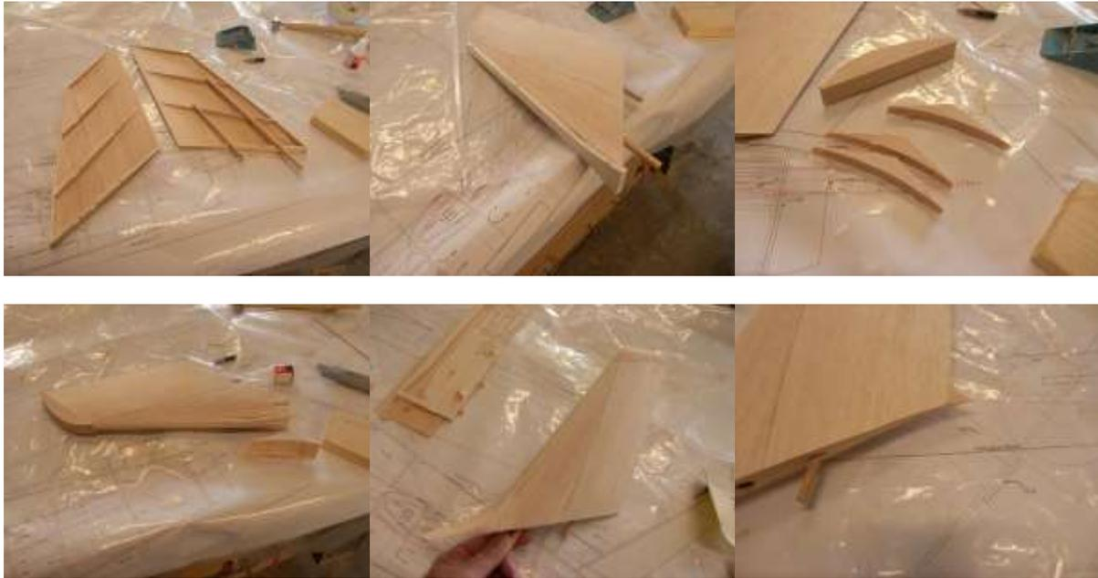
Place dowels , cut dowels to size after test fitting to fuselage
