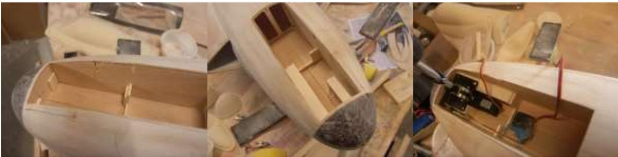
**Front hatch is made in 2 pieces . We used springs and rubber bands for closing , we mount the hinges with fasteners and epoxy, and these parts are not in the kit it is all DIY**
