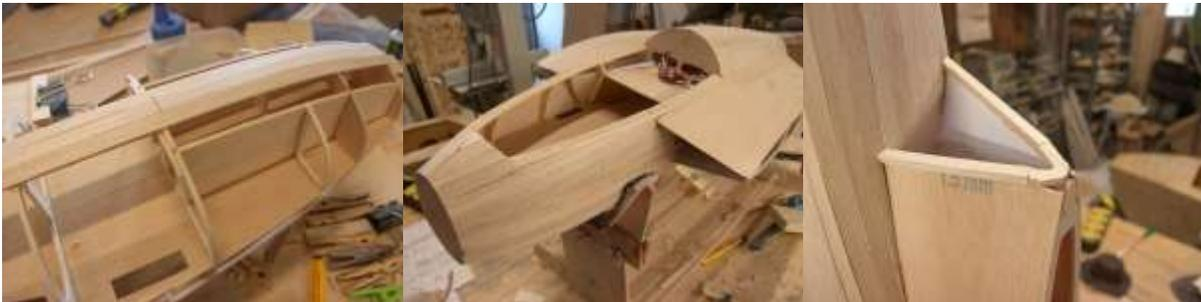
**Clean up at the wing fairings, sand front to Place the nosecone with Dowel.**
