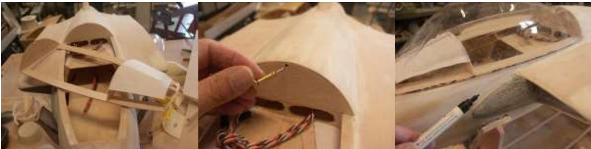
**Glue canopy closing with some scrap balsa to canopy , cut out hatch. And place formers.**
