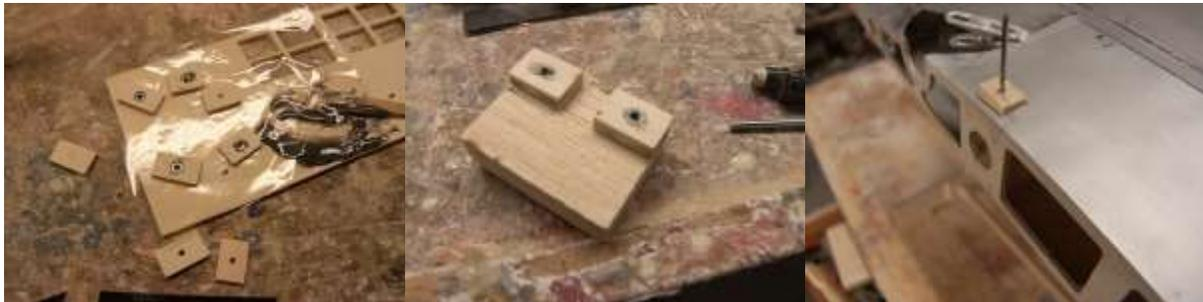
Drill holes into former with a 2,5mm drill take out assembly and drill 4mm, place assembly. Place wings and light drill with a 2mm drill at position , drill joiners with 3mm a few mm, so the M3 will hold the joiner, it is only that it does not slide out you might want to shorten the fasteners.
