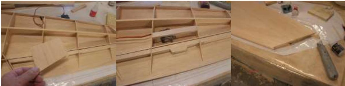
**sand all so there are no high spots and pin down the inner panel to the building board with help from the 6x12 help former for the correct washout, pin down the wing at the X marked points.**
