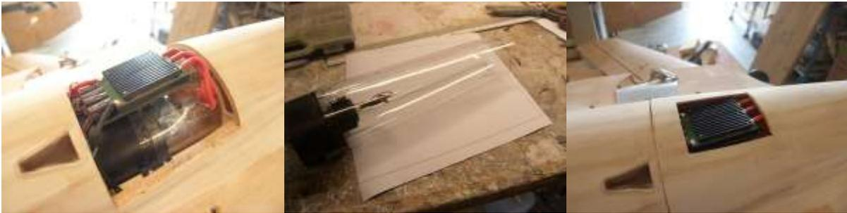
**Place the servo connector plate into the fuselage to F23 so the servo and retract wire can be connect easy, the wing should slide in easy but not loose, if to tight sand joiners.**
