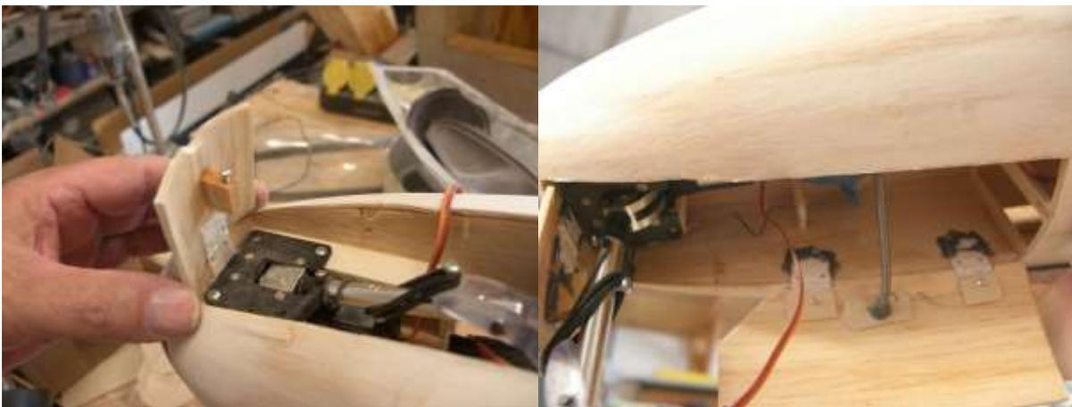
**Cut out main wheel wells in fairings., details for hatch cover are on the drawing, we used thin aluminium, not in kit**
