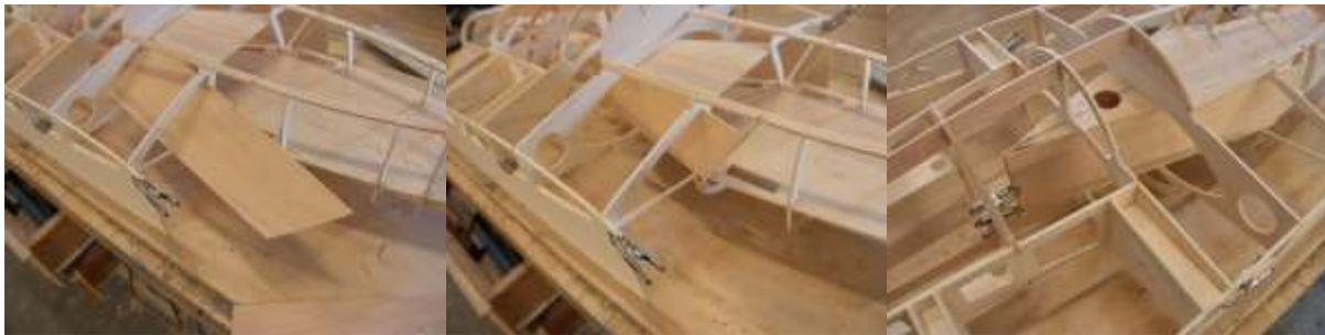
Place duct sheet from stiff paper cut as per plan. Gently push it in and glue to formers
