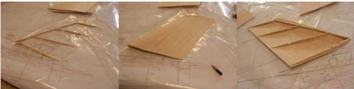
Sheet the ribs with a piece of 1,5mm balsa
