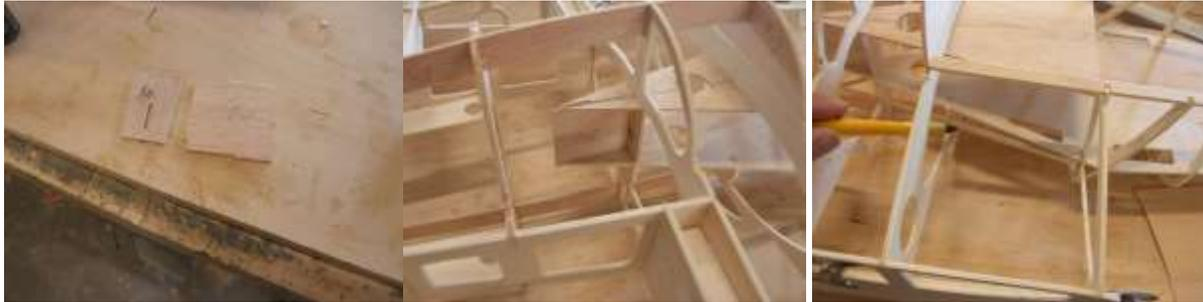
Now place the duct sheeting and lining ,cut as per plan from thick paper in 2 pieces , it can be done in 1 piece note the cut-outs in the paper you might widen them up a bit for easy placing.
