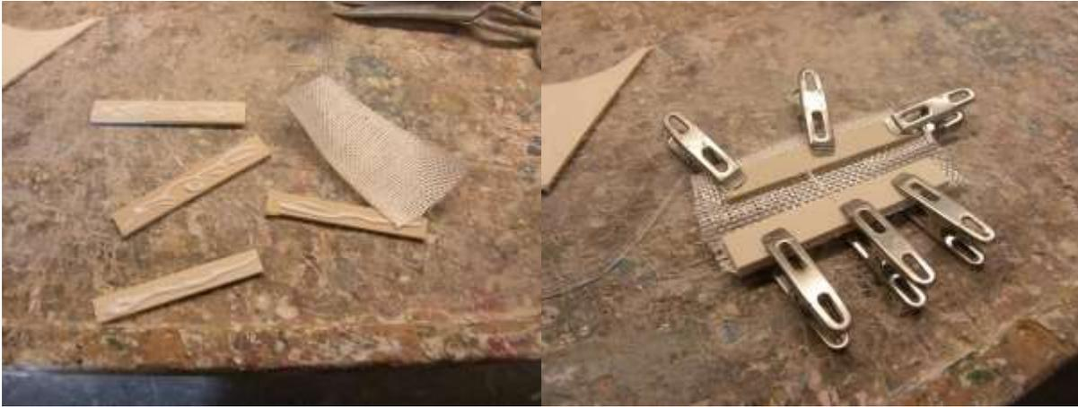
**Glue assembly in fuselage nose section with white glue., place steering servo to floor glue servo to floor use a 1mm steering wire with a z-bend see the drawing**
