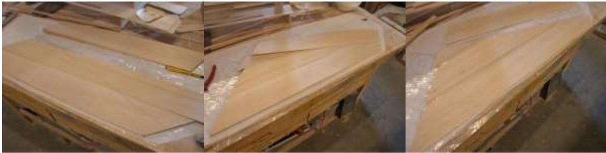
**Take out all parts that are needed for the wings and clean them up with a sanding block from the small holding tabs.**
