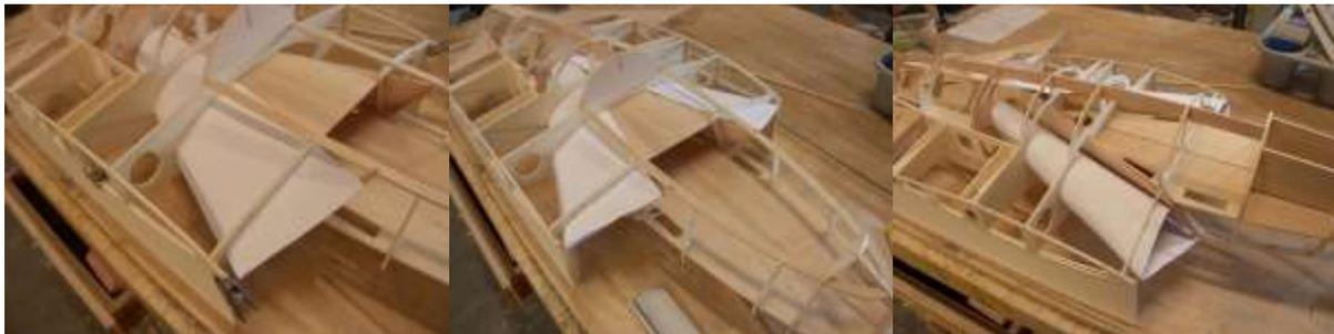
When done place scrap 6x12mm balsa on the intake lips place 3x balsa on the ducts for strengthening as per plan and sand flush to take fairing sheeting.
